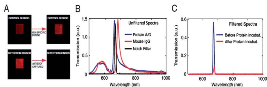
**Fig. 2** (a) Optical images of nanohole arrays functioning as control and detection sensors. The detection sensor appears visibly darker when a monolayer of biomolecules is formed on its surface. (b) Transmission spectra of a notch filter and before (protein A/G) and after (mouse IgG) specific binding of mouse IgG antibodies. (c) Same spectra as in (b), but with the notch filter in place. Figure reprinted with permission from the National Academy of Sciences.<sup>4</sup>
