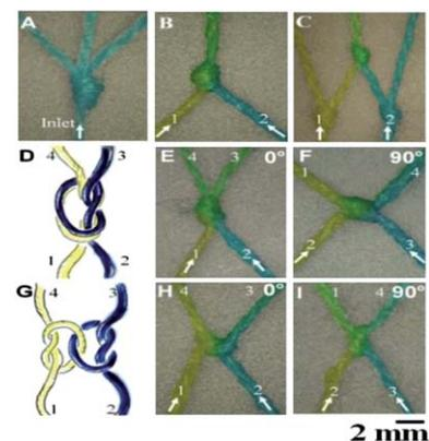
**Fig. 1** Various knots with different topologies used to mix yellow and blue dyes in cotton yarn. Figure reprinted with permission of the Royal Society of Chemistry from Safavieh *et al.*<sup>2</sup>
