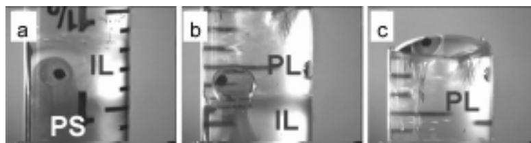
**FIG. 2.** Video images of the magnetically driven conformal coating process in a gradient composed of 10% HEMA–MMA in PEG (polymer solution, PS), a PEG intermediate layer (IL), and a PBS precipitation layer (PL). (a) Bead as it deforms the PS–IL interface and entrains polymer ( $t = 5$  s); (b) bead as it passes through the IL–PL interface ( $t = 7$  s); (c) precipitation of the coating in the PL ( $t = 15$  s)
