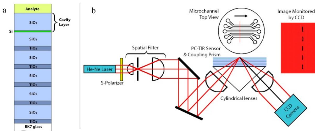
Figure 2. PC-TIR sensor: (a) Photonic crystal structure with open cavity. (b) Schematic diagram of a PC-TIR experimental setup with image of resonant dark lines captured by the CCD camera.
