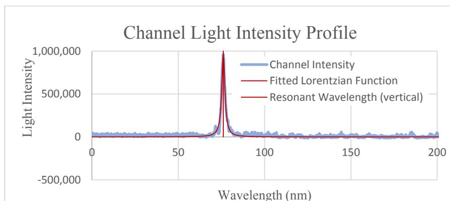
Figure 3. Light intensity profile of a channel after subtraction from the reference channel. The peak was the dark line in the channel image. To find the center of the dark line, the profile was fit to the Lorentzian function (equation 1).
