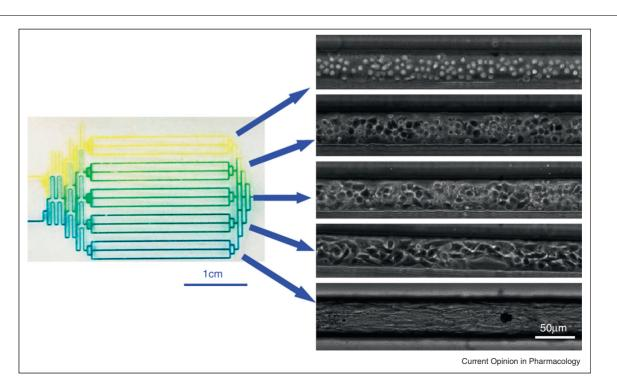
Example of a microfluidic organ-on-a-chip for tissue culture. The top view of the device (left) shows an array of parallel microfluidic channels, which can be loaded with different cells, growth factors, or drugs (here visualized with different food dyes). The phase contrast images on the right exemplify the results of different cell culture conditions (rat cardiofibroblasts) on the same chip.
