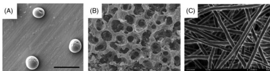
**Figure 1.** SEM images for solid peroxide-incorporated biomaterials. (A) Core-shell  $\text{H}_2\text{O}_2$ -poly(2-vinylpyrrolidone) microspheres. (Li *et al.*<sup>15</sup> Copyright 2012 with permission from Elsevier.) (B) 5%  $\text{CaO}_2$ -poly(D,L-lactide-co-glycolide) scaffolds. (Oh *et al.*<sup>3</sup> Copyright 2009 with permission from Elsevier.) (C) 10%  $\text{CaO}_2$ -polycaprolactone electrospun nanofibers. (Wang *et al.*<sup>33</sup> Copyright 2011 American Chemical Society.)
