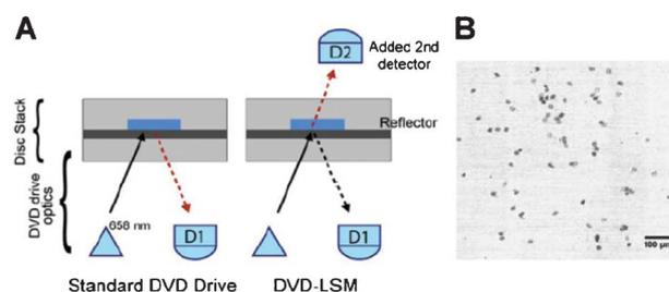
**Fig. 1** (A) A comparison between a standard DVD drive and the DVD-Laser Scanning Microscope (DVD-LSM) mode of operation. In the DVD-LSM a second detector (D2) was placed above the disc. (B) CD4+ cells captured on the surface of the DVD coated with anti-CD4 antibodies, using the DVD-LSM. Adapted from Ramachandraiah *et al.*<sup>3</sup>
