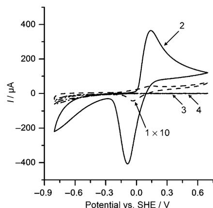
**Figure 3.** Whole-cell CVs (scan rate 10 mV s<sup>-1</sup>) of *S. loihica* measured in the absence (trace 1) and presence (trace 2) of  $\alpha$ -Fe<sub>2</sub>O<sub>3</sub> colloids (7.5 mM). Trace 3: CV of the  $\alpha$ -Fe<sub>2</sub>O<sub>3</sub> colloidal solution lacking cells, trace 4: CV of the cell-free supernatant obtained after the CV measurement of *S. loihica* in the presence of colloids. The waveform in trace 1 was expanded in the  $y$ -axis direction by a factor of 10.
