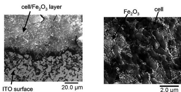
**Figure 2.** SEM images of the surface of the ITO electrode (seen from above) after 28 h of current generation in the presence of  $\alpha$ -Fe<sub>2</sub>O<sub>3</sub> colloids.
