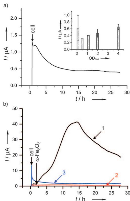
**Figure 1.** a) Current  $I$  versus time  $t$  measurements of microbial current generation for *S. loihica* on an ITO electrode. Inset: the dependence of the steady-state current on  $OD_{600}$ . b)  $I$  versus  $t$  curves in the presence (trace 1) and absence (trace 2) of  $\alpha$ -Fe<sub>2</sub>O<sub>3</sub> colloids (7.5 mM). The effect of iron citrate (7.5 mM) is shown in trace 3. No agitation was made during measurements.
